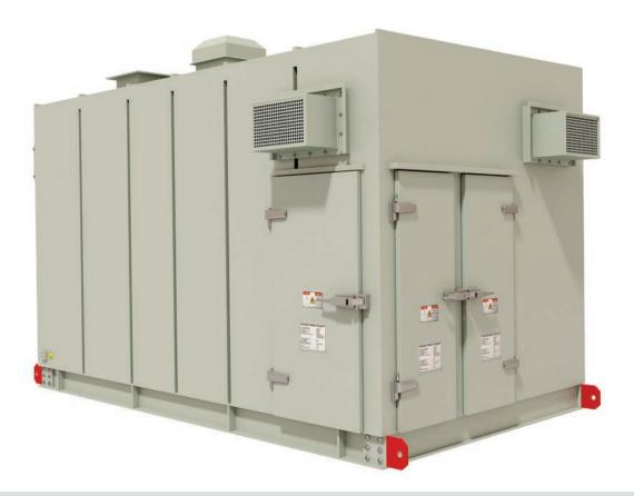
Generator Circuit Breaker cubicles are medium voltage metal enclosed cubicles containing a Generator Circuit Breaker, disconnect switches, earthing switches, instrument transformers and surge protection devices for isolation, synchronization and protection of power systems.
